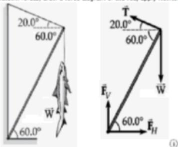
Part 3 of 4 - Analyze Tension between cable & rod
