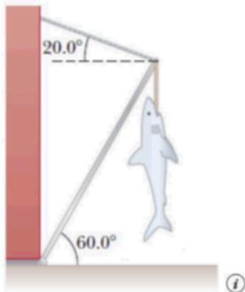
(a) Calculate the tension in the cable between the rod and the wall, assuming the cable is holding the system in the position shown in the figure.
