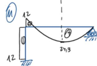
$$\begin{aligned} M_{\max} &= M_A + V_A \times d - 15 \cdot u - \frac{u^2}{2} \\ &= 12 + 33 \times 2,20 - 7,5 \times 2,20^2 \\ &= 24,3 \text{ kNm} \end{aligned}$$
