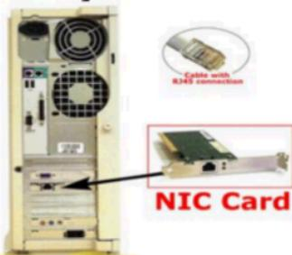
Most of the MAC addresses are assigned by the manufacturer of the Network Interface Cards (NIC), where they are stored in hardware. It is constituted by a sequence of 48 bits (MAC-48)
