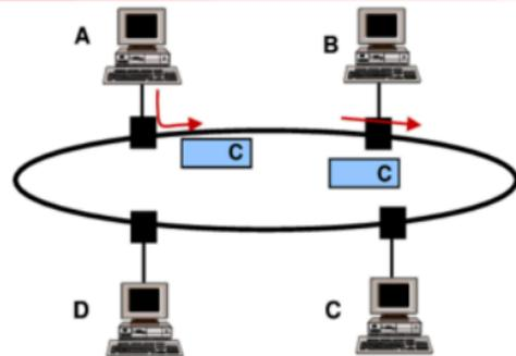
A sends one frame to C. The frame passes through B. This node ignores the frame.
