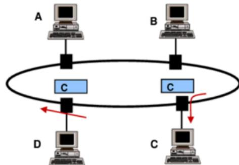
In C the frame is copied. This frame continues to circulate in the ring up to A where it is removed.
