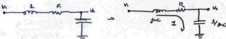
$$\frac{V_0}{V} = \frac{j/\omega C}{\frac{1}{\omega C} + j\omega L + R} = \frac{1}{1 - j\omega^2 LC + j\omega RC} = T(\omega)$$
