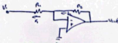
$$A_{dC} = 200 \text{ 000} \rightarrow R_2 = 200 \text{ k}\Omega$$
