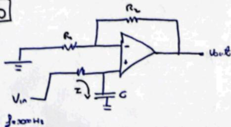
$$\begin{array}{l|l} R = 5300 \Omega & R_1 = 10 \text{ k}\Omega \\ C = 10 \text{ nF} & R_2 = 22 \text{ k}\Omega \end{array}$$
